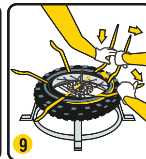
9 These motorcycle tire levers will help the bead to descend into the rim well and will allow you to finish fitting easily with others 3/4 tire levers.
