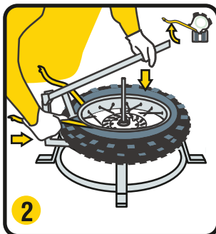
2 Lubricate the flat side of 2 motorcycle tire levers and insert them approximately 5 cm apart between the tire bead and the rim.
