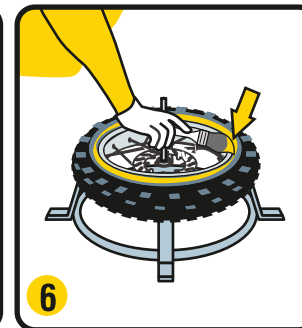
6 Lubricate the 2 nd bead on its 2 surfaces (inner and outer) and then insert it partly on the rim.
