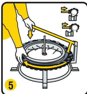
5 Slide the tire cover/mousse assembly on the rim towards the outside.
