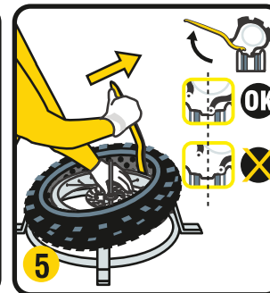
5 Insert the 1 st bead on the rim, taking care to push the mousse as far as possible into the rim well. If necessary, finish fitting using a tire lever.
