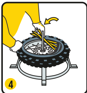
4 Finish removing the 1st bead: lubricate the bottom part of mousse that is in contact with rim.
