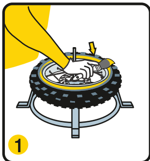
1 Make sure the tire and mousse is cool before removing it. Disengage and liberally lubricate the tire beads.
