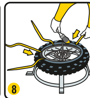
8 About 30cm from the fixed first tire lever, slide a tire lever between the rim edge and the tire bead with the flat side stopped against the rim wall.
